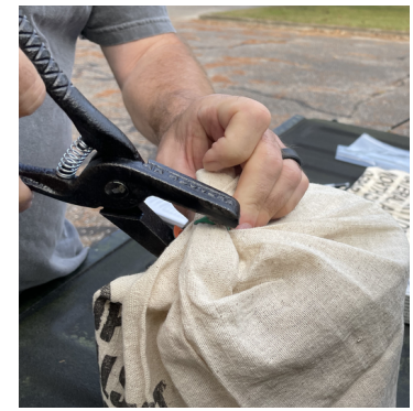
6. Crimp the metal tag to seal the cloth bag
